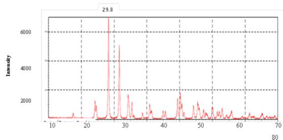
Figure 5: shows X-ray diffraction patterns of ZrO<sub>2</sub> nanoparticles and its intensity.
