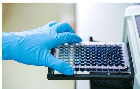
Figure 1: ELISA reader for measuring the samples optical density
